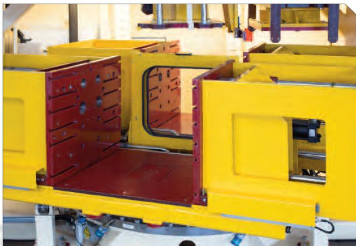
► Spara anime cold-box SPF 60 - Core making machine SPF 60
